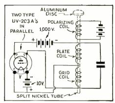
Fig. 2. Circuit of the set-up shown in Fig. I.
